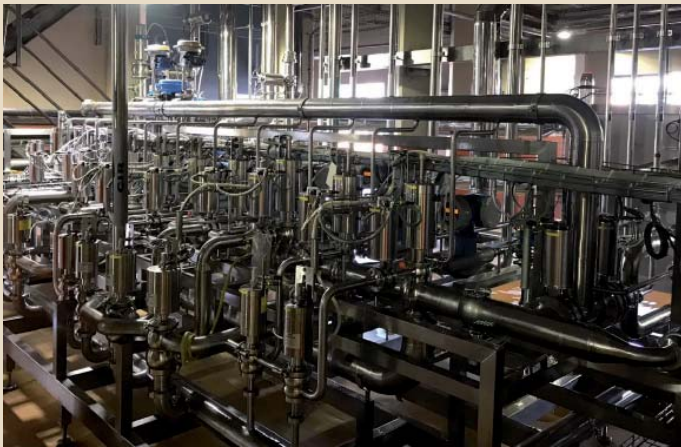
Fig. 5 Mixing system capable of incorporating thirteen liquid product streams
